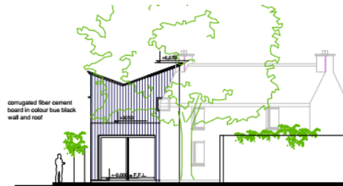
East Rear Elevation - back garden
