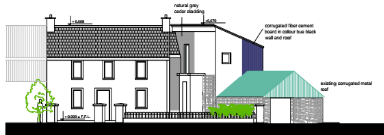
North- West elevation View from Youghal Road
